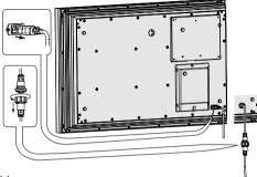
**2** Remove the screws on the back of the cabinet, and then remove the terminal covers.
